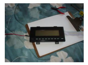
Replace the display and control board (making sure to carefully route the LCD red/black wire harness through the circular hole in the control board). Reconnect the red/black harness to its connector.
