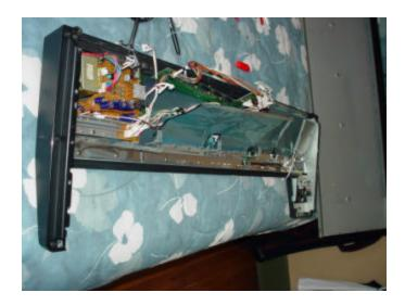
You can now remove the foil blankets by unscrewing them from the attachment plate at the lower edge of the synth case. Remove both blankets and related screws, noting where the screws came from and move them to a safe place. There is a smaller third foil blanket on the left side of the synth that does not need to be removed. Leave those screws in place.
