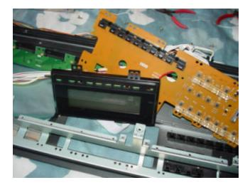
Remove the LCD assembly from the case. It will have a grey ribbon cable and the red/black wire harness still attached. Be careful with these when moving the unit around. Be careful not to scratch or otherwise harm the front of the display area. Set the display assembly face-down on a soft area and remove the four mounting screws holding the LCD circuit board to the plastic face plate. Remove the LCD circuit board from the plastic face plate.
