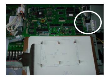
Repeat the process for the DM2 System board located on the left-hand side. This is the bigger board. There is a short cable that connects DM1 and DM2 in the upper right-hand corner of the DM2 board – you can leave this cable attached to DM2 but disconnect all others. Document everything, and remove the board to a safe location.
