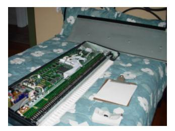
Begin by removing the DM1 System Board on the right-hand side of the synth. Remove and document the locations of the 6 anchor screws and all cables and wire harnesses. Notice the example marker lines on the cable and socket circled below to show cable orientation. Remove the board and place it (along with the documentation and screws) in a safe, out-of-the-way place.
