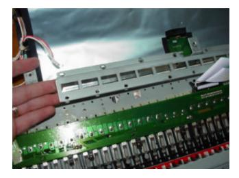
You now need to remove the keybed assembly. There are only four black screws holding the keybed to the metal frame, one on each corner. Remove these screws. Also, remove the aftertouch ribbon cable by carefully pulling up on the lock bracket located on a small circuit board on the upper left-hand side of the keybed. Carefully slide the aftertouch ribbon out (noting the direction it goes in) remove any other wire harnesses connected to the keybed and move the entire keybed to a safe location.
