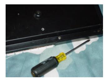
Remove all of the screws holding the bottom plate. There are quite a few, and it will make things easier to keep track of if you use the following trick. Make a large drawing of the bottom of the synth on a piece of paper. Make note of the location of all screws on this drawing. When you remove a screw, tape that screw to your drawing so that you can make sure to keep track of exactly what screw goes where. You can also use a digital camera for this type of documentation.
